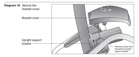
20. **Attach the bracket cover.** Diagram 16. Take the following steps to attach the cover over the upright support bracket.
